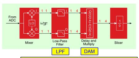
The 16 samples per transmitted bit are first reduced to 4 and later back to 1.
