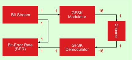
Modulated signal has 16 samples per transmitted bit.
